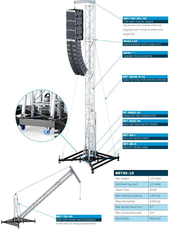
To lift the tower, a special tower erecting part can be attached to the central base, this part acts as a lever to bring the tower into its final position.
