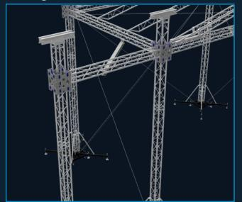
For the SDR30 roof PA Wings are available and extend the width of the SDR roof by ~3,5 meters on each side. The PA Wing itself is 3 meters in width. The maximum load is 1.000 kg CPL on each side.
