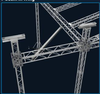
To give horizontal support to the PA-Wings NEXT chooses to use small "H" steel profiles as diagonal support for the PA-Wings. The beams are small and will therefore need small "holes" in the side walls, the other advantage and main reason is the additional pick-point for the PA cluster.
