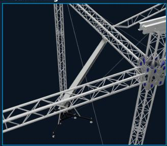
To give horizontal support to the PA–Wings NEXT chooses to use small "H" steel profiles as diagonal support for the PA–Wings.
