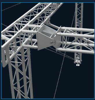
To connect the PA wings to the ARC30 roof, a different corner must be used at the front legs. In addition, a swivel piece must be added to distribute the forces correctly.
